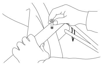
Align the screw hole on the leg pipe with the screw hole on the armrest so that a screw can sit straight in the hole. First turn the screw a few times with your hand, not with the screw driver, to temporarily fix it. Do the same with the opposite side.
