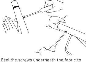
Feel the screws underneath the fabric to ensure they go through the pipe, check the tension of the seating fabric, and fully tighten the screws.
