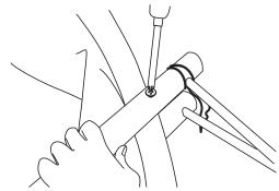
After you have tightened temporarily all the four screws, tighten them with the screw driver until they penetrate into the leg pipe
