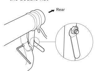
Using a screwdriver and the supplied allen wrench and spanner, tighten the pre-tightened screw and the bottom of the double nut until there is no gap.
