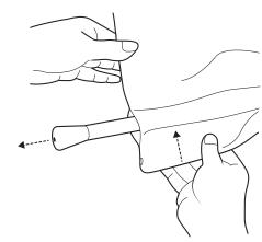
Pull out the seat pipes from the seating fabric.
