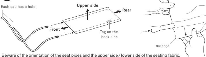
(Make sure that the tag and the care label are on the lower side of seating fabric.) Push the seat pipes firmly into the seating fabric, and at last place the edge of the seating fabric over the seat pipes. (The seat pipes are completely hidden.)
