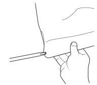
There is a hole on the front of the seating fabric for attaching a screw. Use a Allen wrench or similar method to spread the hole where the screw is inserted.
