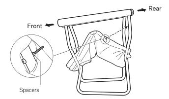
Pass the screw through the seat pipe before attaching the spacer.
