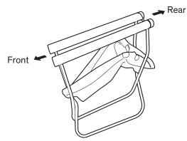
Position the seat so that the rear seating fabric is on the higher arm and the front seating fabric is on the lower arm.
