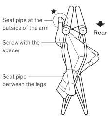
Adjust the seat pipe to position its ★ section at the outside of the arm and the rear seat pipe between the legs, and pass the screw through the leg.
