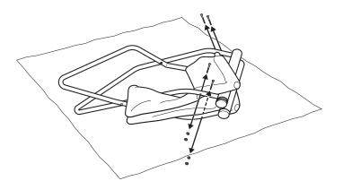
Work with a rug on the floor and lay the body of the chair. Remove screws from the body and disassemble the seating fabric and body.
