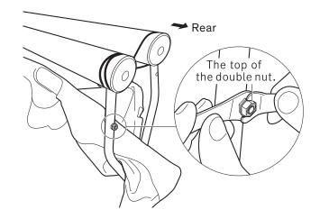
Hold the bottom of the double nut with a spanner so that it does not move, and turn the top of the double nut with another spanner to tighten it.
