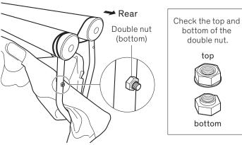
Pre-tighten the bottom of the double nut on the screw tip. (Rotate by hand about 2 turns)
