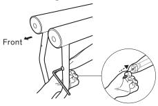
While holding the seating fabric, pass the screw through the seat pipe and tighten it with a allen wrench, so that the seat pipe is positioned on the edge of the seating fabric.
