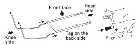
Insert the pipe into each pipe hole of the new seating fabric in the direction shown above.
