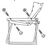
Assemble the chair legs and the new seating fabric with the pipes inserted by using the screws.
